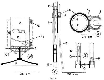
Water leveller. W, reel and reservoir assembly; X, section of slide and tube holder; Y, levelling staff; Z, feet of staff. A, drum; B, flange; C, stand; C<sub>1</sub>, brace; D, reservoir; E, tube; E<sub>1</sub>, slack tube; F, upper portion of the staff; G, lower portion; H, connecting piece; I, slide; J, tube holder; K, clamp; L, slot for tube; M, measuring tape; N, protecting cap; O, slot for tape; P, guide; Q, datum mark.
