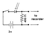
FIG. 2. Circuit diagram for the photodiode. See text for explanation.
