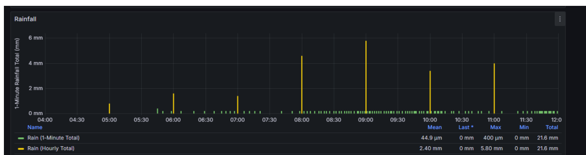
FIGURE 7. Rainfall record for 2 January 2024 for Dale Fort. The image shows a screenshot from an automatic weather station. The green lines show amounts per minute while the yellow lines show hourly totals (for the hour starting where the line is plotted).
